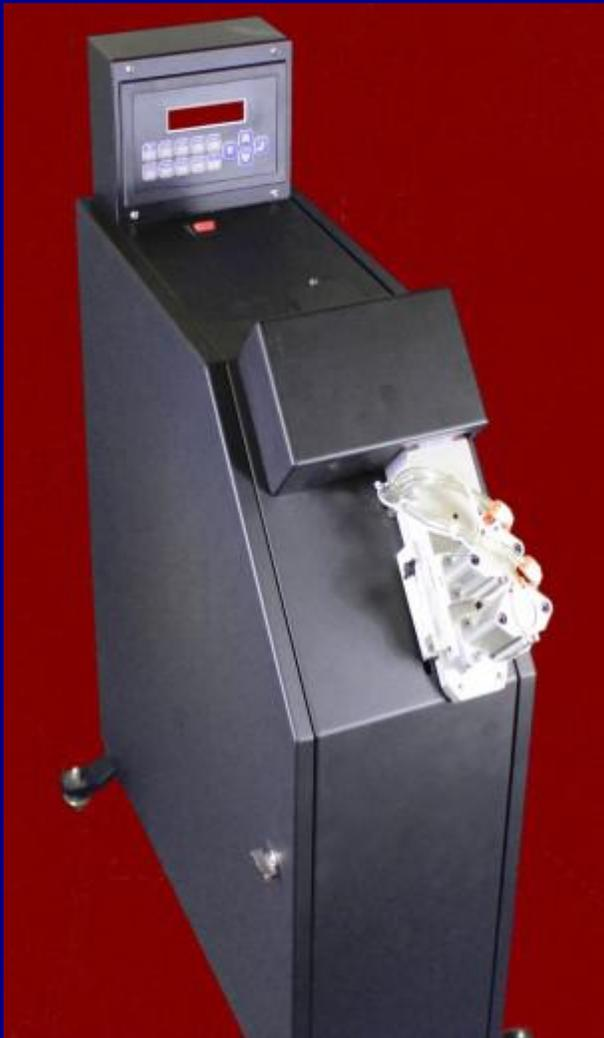
The Auto-Stic machine was developed to be used with Stic-N-Pic®\*\* strips for a faster and more consistent application.
