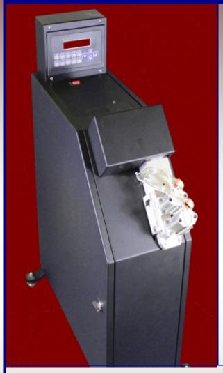
The Auto-Stic machine was developed to be used with Stic-N-Pic®\*\* strips for a faster and more consistent application.
